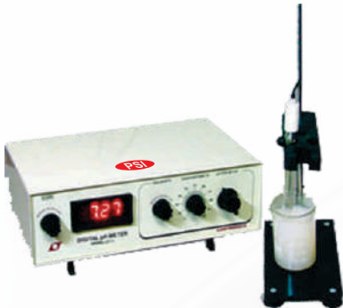
PSI -056 : PH METER WITH COMBINED ELECTRODE
